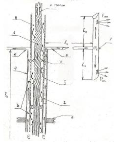
Figure 3 - Basic construction diagram of the turbine type H - Rotor
