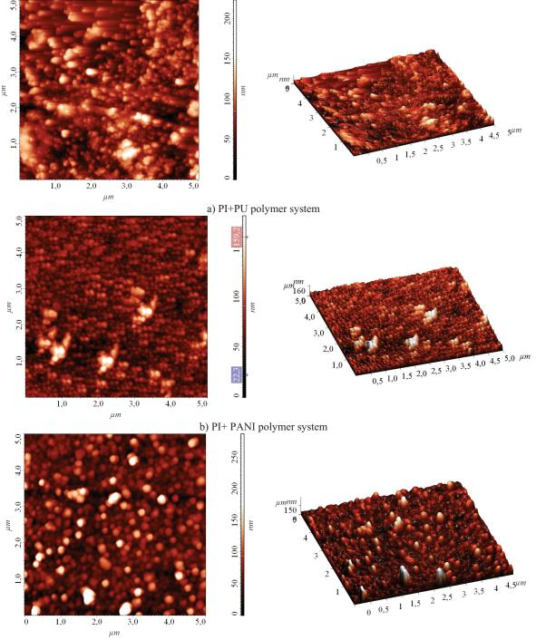
c) PI+PU+PANI polymer system **Figure 1 -** AFM image of the composite polymer systems
