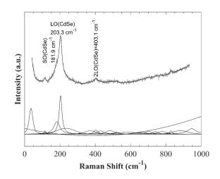
Figure 7 – Raman spectrum of sC. Raman peak positions corresponding to LO and SO phonon modes of CdSe nanocrystals are indicated.
