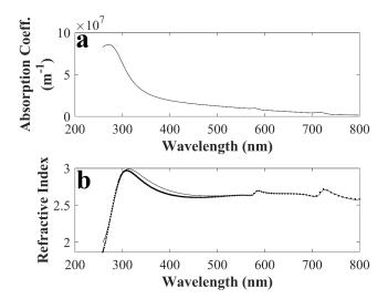
Figure 4 – Absorption coefficient (a) and refractive index (b) of bulk CdSe. At (b), line and dots correspond to refractive index produced from the study of Ninomiya and Adachi [19], and K-K transformation, respectively.
