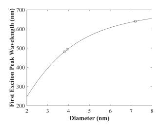
**Figure 6** – First peak wavelength versus diameter for CdSe nanocrystals in glass. Circles point out diameters/peak wavelengths for sC, sD and as received.  $E_g, m_e^*, m_h^*$  and  $\varepsilon$  are taken as 1.74 eV, 0.12m<sub>0</sub>, 0.90m<sub>0</sub> and 9.29, respectively. Here,  $m_e^*, m_h^*$  and m<sub>0</sub> are electron effective mass, hole effective mass and electron rest mass, respectively.
