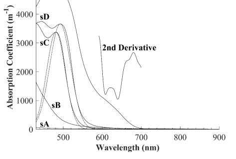
Figure 5 – Optical absorption spectra of CdSe nanocrystals in glass. Sampels; sA: melted, sB: 531°C-15 days, sC: 531°C-46 days, sD: 531°C-75 days, and sE: as received. Dash-dotted lines show Gaussian curves for sC and sD. Second derivative of absorption of sE is indicated.
