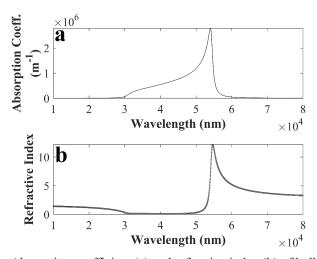
**Figure 3** – Absorption coefficient (a) and refractive index (b) of bulk BaF<sub>2</sub>. At (b), gray line and black dots correspond to refractive index produced from the classical dispersion theory and K-K transformation, respectively.
