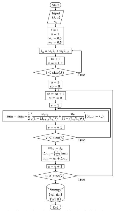
Figure 2 – Flowchart of computation of the refractive index change.
