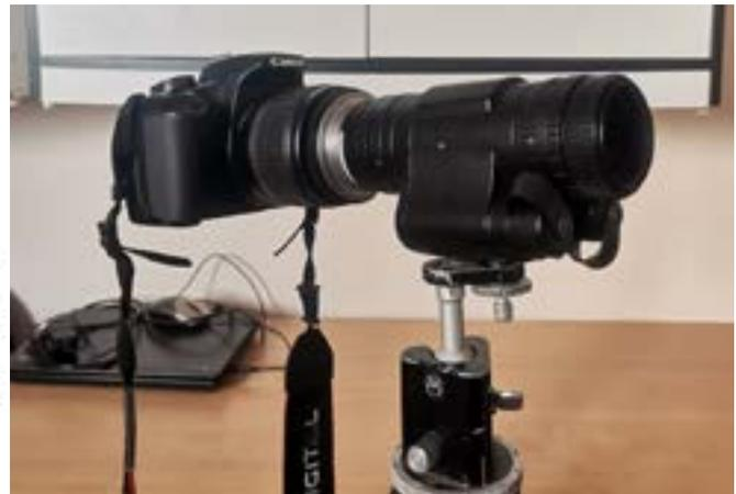
**Figure 4** – General view of the MPN-8KM device – on the left (1 – eyepiece with eyecup; 2 – lens; A – lens focusing unit; 3 – infrared filter; 4 – battery pack), on the right is a device with a CANON-600D camera.
