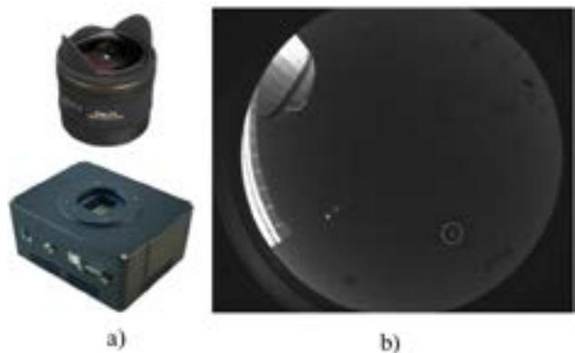
**Figure 3** – a) Fisheye lens (top) and ST 3200 ME matrix;
