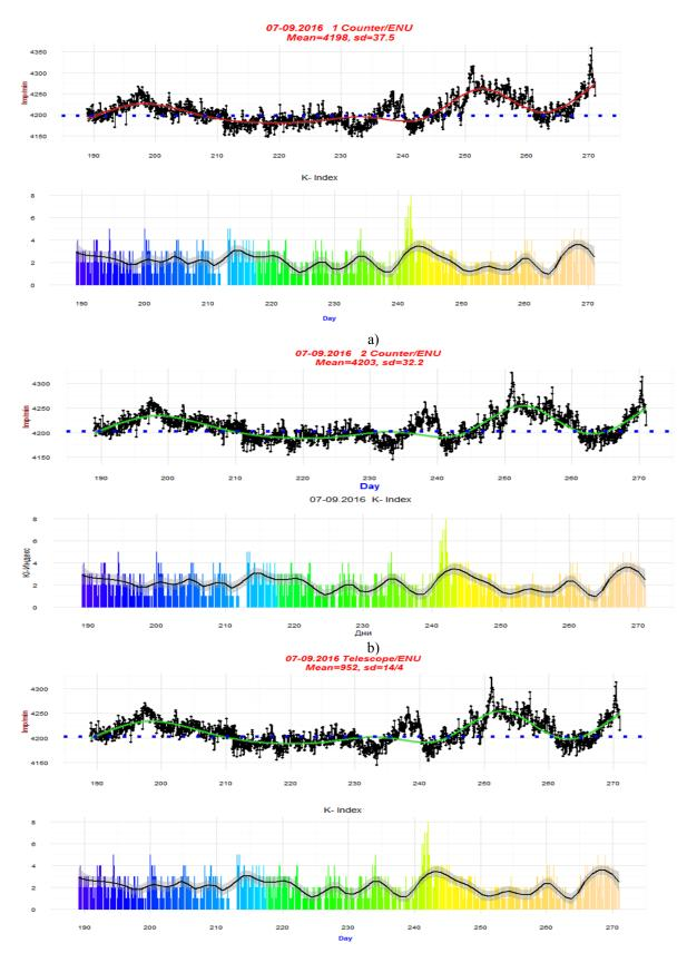
**Figure 6** – Temporal variation of general ionizing component of secondary cosmic rays flux in three channels of the CARPET detector and the dynamics of variation of K-index - the geomagnetic activity
