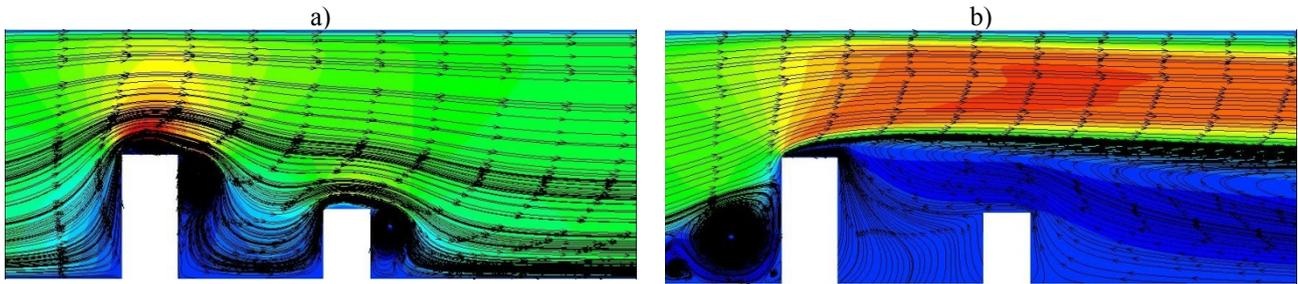
**Figure 7** – The horizontal velocity components of ( $v=0.1$  m/s) of flow around the technogenic obstacles with streamlines, which are calculated by using the DNS for the distance  $l = 31$  (m) at different times (at  $t=0.001$ ,  $t=2$ ).
