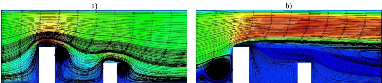
**Figure 9** – The horizontal velocity components of ( $v=0.1$  m/s) of flow around the technogenic obstacles with streamlines, which are calculated by using the DNS for the distance  $l = 35$  (m) at different times (at  $t=0.001$ ,  $t=2$ ).
