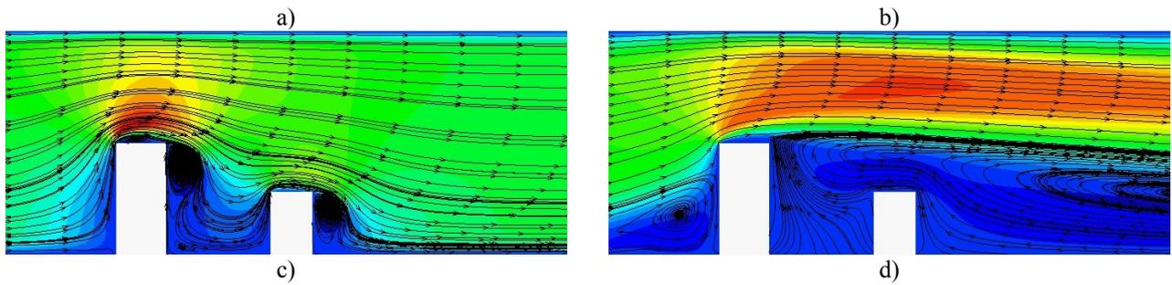
**Figure 4** - The horizontal velocity components of ( $v=0.1$  m/s) of flow around the technogenic obstacles with streamlines, which are calculated by using the DNS for the distance  $l = 25$  (m) at different times (at  $t=0.001$ ,  $t=2$ ).
