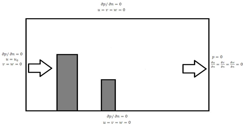
**Figure 1** – Scheme of boundary and initial conditions.
