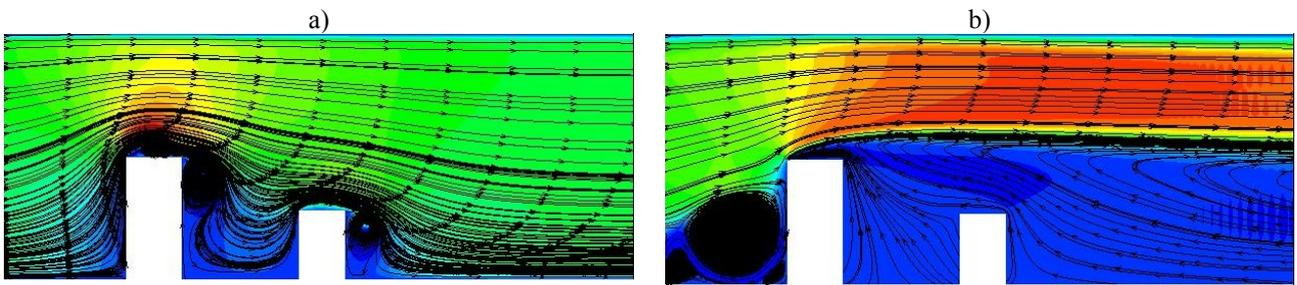
**Figure 5** - The horizontal velocity components of ( $v=0.2$  m/s) of flow around the technogenic obstacles with streamlines, which are calculated by using the DNS for the distance  $l = 25$  (m) at different times (at  $t=0.001$ ,  $t=2$ ).
