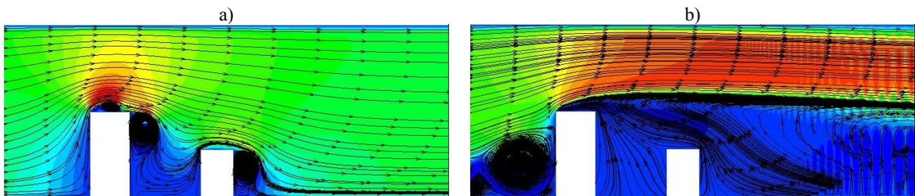
**Figure 3** - The horizontal velocity components of ( $v=0.2$  m/s) of flow around the technogenic obstacles with streamlines, which are calculated by using the DNS for the distance  $l = 20$  (m) at different times (at  $t=0.001, t=2$ ).
