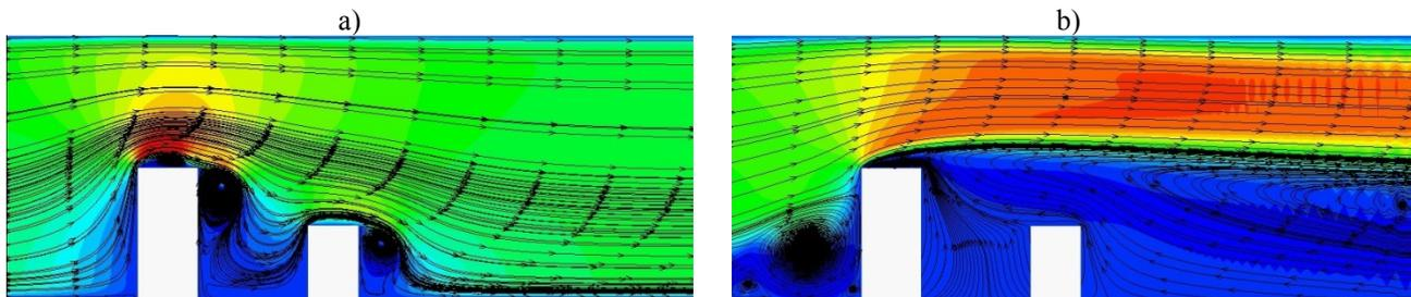
**Figure 2** - The horizontal velocity components of ( $v=0.1$  m/s) of flow around the technogenic obstacles with streamlines, which are calculated by using the DNS for the distance  $l = 20$  (m) at different times (at  $t=0.001, t=2$ ).
