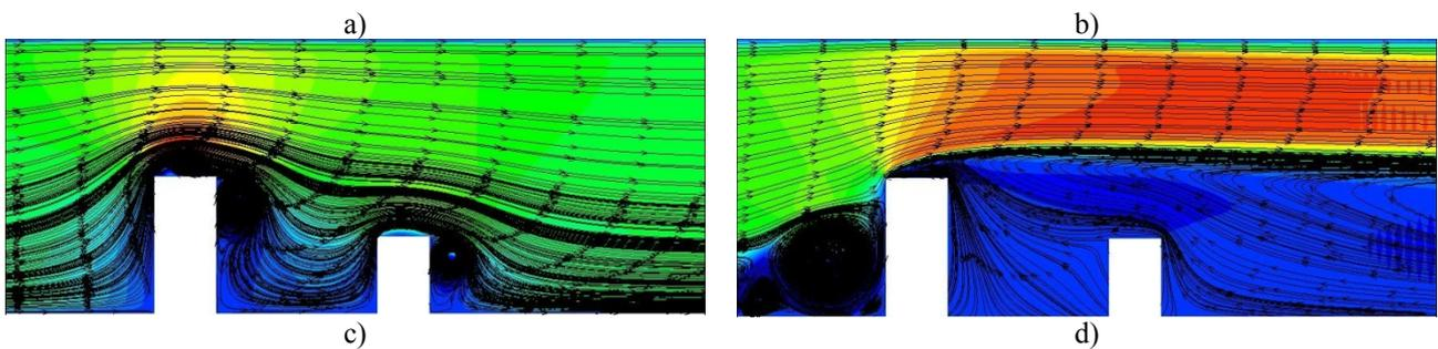
**Figure 8** – The horizontal velocity components of ( $v=0.2$  m/s) of flow around the technogenic obstacles with streamlines, which are calculated by using the DNS for the distance  $l = 31$  (m) at different times (at  $t=0.001$ ,  $t=2$ ).
