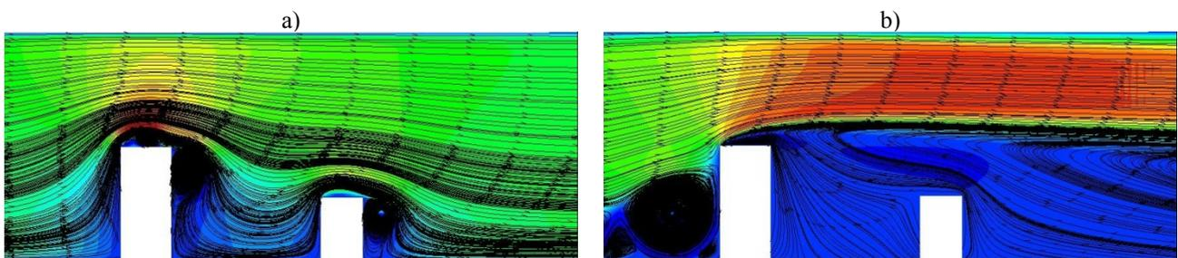
**Figure 10** – The horizontal velocity components of ( $v=0.2$  m/s) of flow around the technogenic obstacles with streamlines, which are calculated by using the DNS for the distance  $l = 35$  (m) at different times (at  $t=0.001$ ,  $t=0.5$ ,  $t=1$ ,  $t=2$ ).
