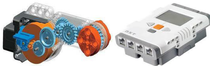
Figure 1 – Main elements of the robot. Servomotor and managing elements
